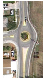
Lack of deflection
