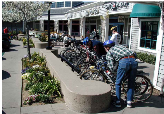
Figure 11 - Bicycle parking should be separated from pedestrian walkways and convenient to the building entrance (image courtesy of pedbikeimages.org / Dan Burden)
